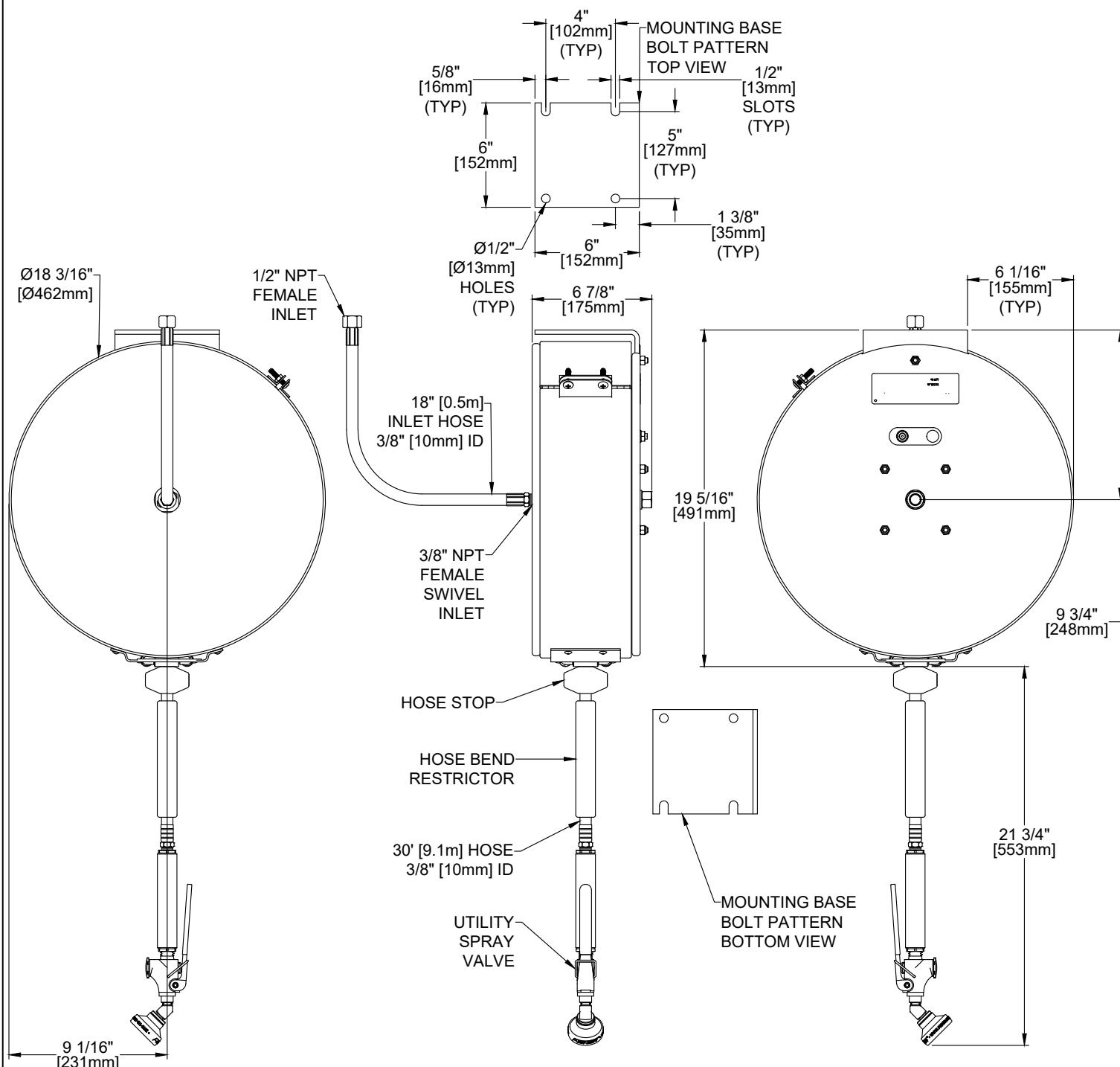
PRODUCT SPECIFICATIONS: CAFE REEL RINSE, COVERED WHITE POWDER COATED STEEL, CEILING MOUNT, 30' HOSE X 3/8" ID, 2.65 GPM @ 80 PSI UTILITY SPRAY VALVE, 18" INLET HOSE X 3/8" ID, 1/2" NPT FEMALE INLET
