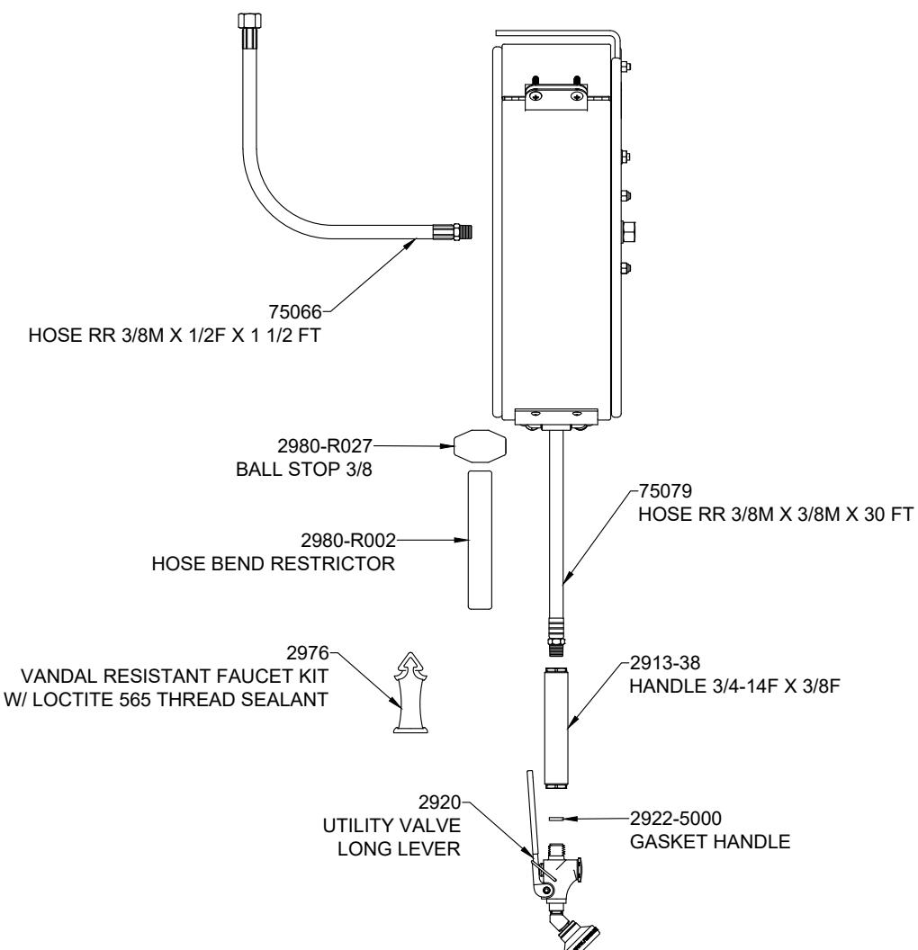
PRODUCT SPECIFICATIONS: CAFE REEL RINSE, COVERED WHITE POWDER COATED STEEL, CEILING MOUNT, 30' HOSE X 3/8" ID, 2.65 GPM @ 80 PSI UTILITY SPRAY VALVE, 18" INLET HOSE X 3/8" ID, 1/2" NPT FEMALE INLET
