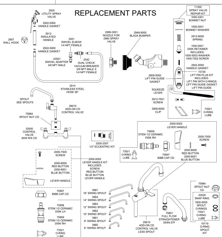
PRODUCT SPECIFICATIONS: 8" ADJUSTABLE WALL MOUNT FAUCET, QUARTER TURN CERAMIC DISC CARTRIDGES W/ CHECK STEMS, LEVER HANDLES, ADD-ON FAUCET, SWING SPOUT W/ FULL FLOW STREAM STRAIGHTENER, 36" FLEXIBLE STAINLESS STEEL HOSE, 2.65 GPM @ 80 PSI UTILITY SPRAY VALVE, SWIVEL ELBOW W/ IN-LINE DUAL CHECK VACUUM BREAKER, WALL HOOK, 1/2" NPT FEMALE INLETS
