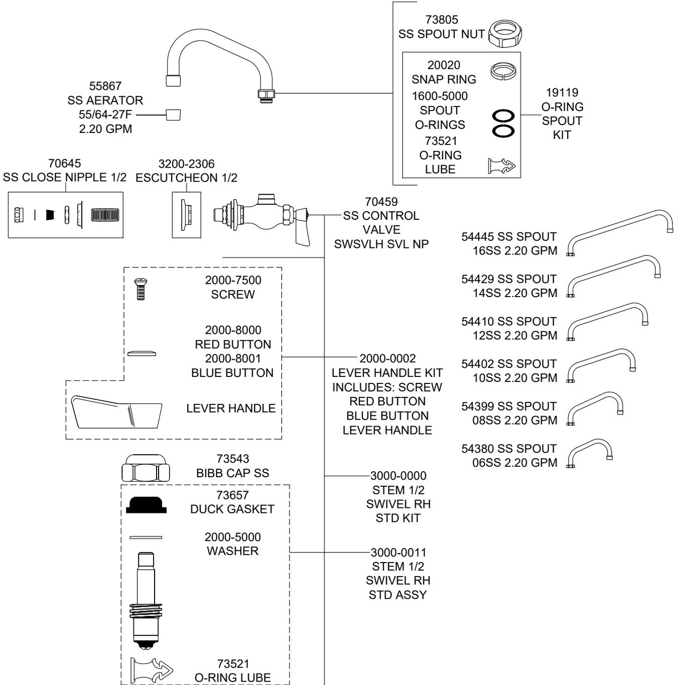
PRODUCT SPECIFICATIONS: STAINLESS STEEL SINGLE WALL / BACKSPLASH FAUCET, QUARTER TURN SWIVEL STEM, LEVER HANDLE, SWING SPOUT W/ 2.20 GPM AERATOR, 1/2" NPT FEMALE INLET, 1/2" NPT MALE NIPPLE INCLUDED
