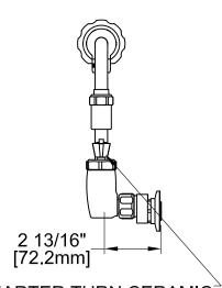
QUARTER TURN CERAMIC DISC CARTRIDGES WITH CHECK STEMS AND COLOR CODED INDEXES
