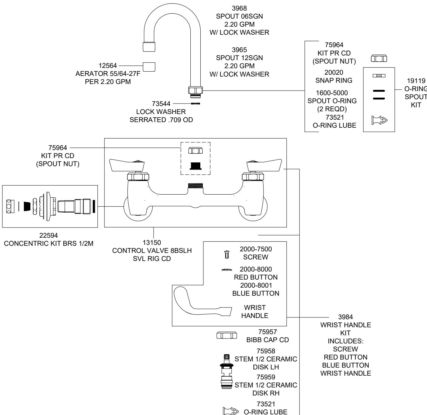
PRODUCT SPECIFICATIONS: 8" BACKSPLASH FAUCET, QUARTER TURN CERAMIC DISK CARTRIDGES W/ CHECK STEMS, WRIST HANDLES, 6" OR 12" SWIVEL OR RIGID GOOSENECK SPOUT W/ 2.2 GPM @ 60 PSI AERATOR, 1/2" NPT MALE INLETS
