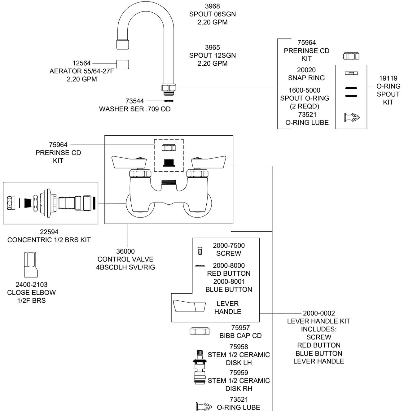
PRODUCT SPECIFICATIONS: 4" BACKSPASH FAUCET, QUARTER TURN CERAMIC DISK CARTRIDGES W/ CHECK STEMS, LEVER HANDLES, 6" OR 12" SWIVEL OR RIGID GOOSENECK SPOUT W/ 2.2 GPM @ 60 PSI AERATOR, 1/2" NPT MALE INLETS W/ CLOSE ELBOW 1/2" NPT FEMALE INLETS
