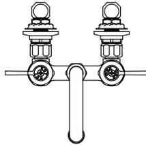
GOOSENECK SPOUT W/ 2.2 GPM AERATOR 55/64-27F, CONVERTS TO RIGID W/ SERRATED LOCK WASHER, INCLUDED
