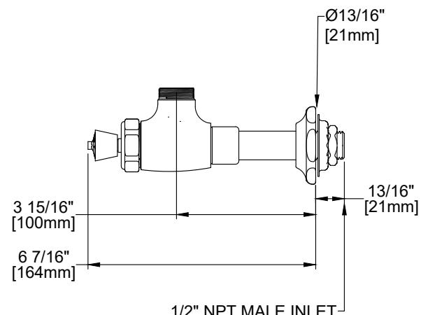
PRODUCT SPECIFICATIONS: CHINESE RANGE CONTROL VALVE, 1/2" X 3 5/8" NIPPLE, QUARTER TURN CERAMIC DISK CARTRIDGE W/ CHECK STEM, LEVER HANDLE, 1/2" NPT MALE INLET
