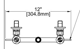
QUARTER TURN CERAMIC DISC CARTRIDGES WITH CHECK STEMS AND COLOR CODED INDEXES
