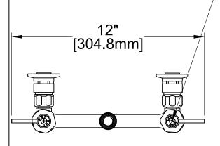
QUARTER TURN CERAMIC DISC CARTRIDGES WITH CHECK STEMS AND COLOR **CODED INDEXES**
