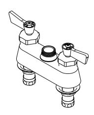
QUARTER TURN CERAMIC DISC CARTRIDGES WITH CHECK STEMS AND COLOR CODED INDEXES
