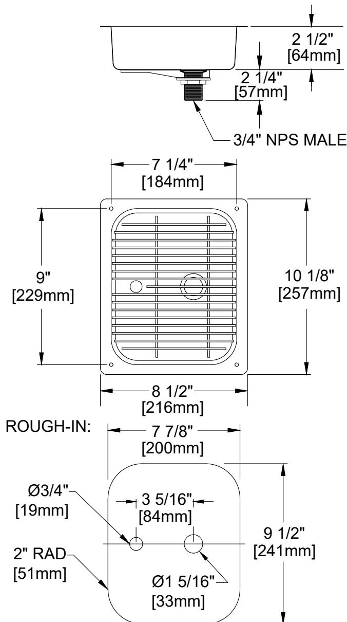
PRODUCT SPECIFICATIONS: STAINLESS STEEL DRAIN PAN W/ ELEVATED PLASTIC DIPPED GRID, & CHROME DRAIN, FOR PEDESTAL GLASS FILLER
