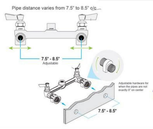
When you see the term "Wall" in our catalog or website what does it mean? It means it comes with the adjustable eccentrics (Eccentrics adjust from 7-3/4" to 8-1/4") to attach the faucet or pre-rinse unit directly to the pipes sticking out of the wall.
